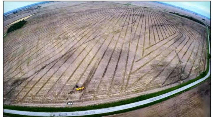
***HDPE pipe has a very favorable strength-to-weight ratio. Plus, for any pattern of tiling the flexibility of the pipe easily accommodates changes in direction.***
